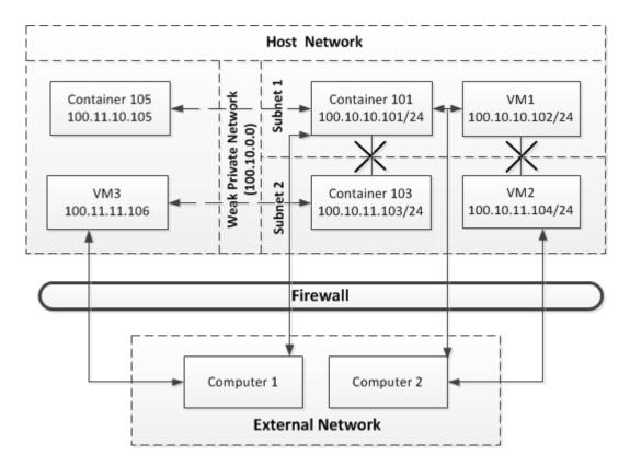
In this example, the private network on the physical server is divided into two subnets: *Subnet 1* and *Subnet 2*. Container 101 and VM1 are connected to Subnet 1, and Container 103 and VM2 are joined to Subnet 2. Container 105 and VM3 do not belong to the private network. Container 101 and VM1 can access each other, but cannot connect to Container 103 and VM2. Container 103 and VM2, in turn, can also access each other, but cannot connect to Container 101 and VM1.
