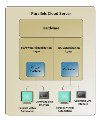
At the base resides server hardware. Next is the Parallels Cloud Server software which is installed directly on the server hardware and does not need any operating system for its functioning. Parallels Cloud Server includes two virtualization layers:
