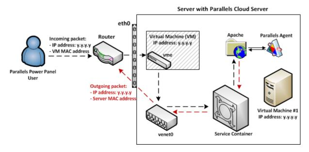
To avoid such problems, you can reconfigure the router to accept packets with the same IP address but different MAC addresses. You can also switch virtual machine's network adapter to the host-routed mode or create an additional network adapter and set it to work in the host-routed mode.
