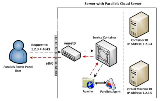
When offline management is enabled, the server keeps ARP and routing entries for host-routed Containers, running host-routed virtual machines, and all stopped virtual machines. In this case, offline management works as follows:
