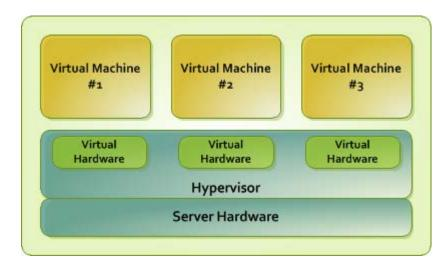
The following diagram shows the basic architecture of hardware virtualization.
