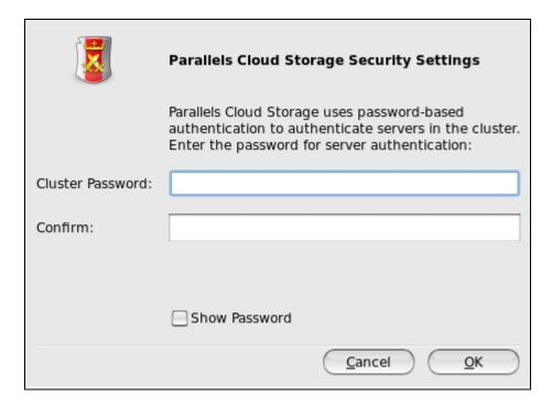
Password-based authentication enhances security, requiring each server to be authenticated before it can be included in the cluster. The password you specify is encrypted and saved to the /etc/pstorage/clusters/CLUSTER\_NAME/auth\_digest.key file on the server.
