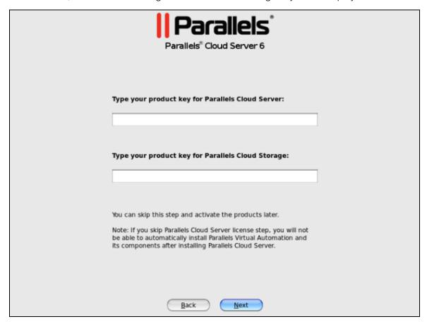
Type the license keys in the fields provided, and click **Next**. You can skip this step and install the keys later. However, if you do not specify the key for Parallels Cloud Server, you will not be able to install Parallels Virtual Automation and its components along with Parallels Cloud Server. For more information about Parallels Virtual Automation, see **Installing Parallels Virtual Automation** (p. 30).
